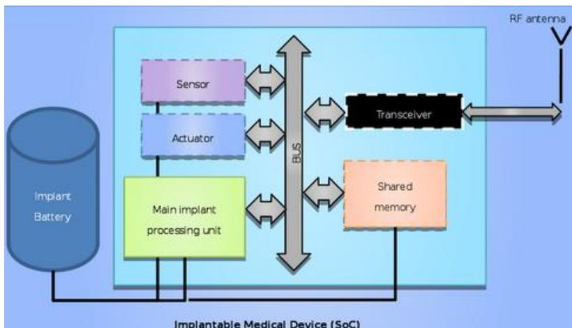
expected to perform their **safety-critical application** on a **limited battery supply** for several years. The treatment-software running on these devices should be **adjustable** (e.g., to update a treatment plan) and monitored remotely, i.e., **secured wireless communication** is required.
